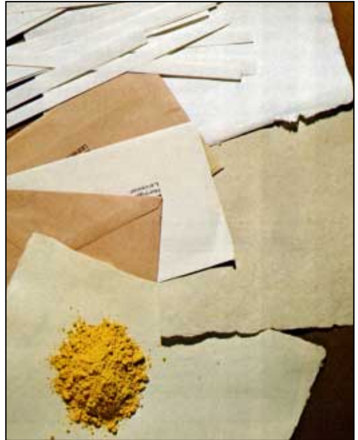
Fig. 5 Paper samples made from dry photocopying paper, (top), white and manilla envelopes, (middle), and white printers' offcuts mixed with yellow powder colour, (bottom).
